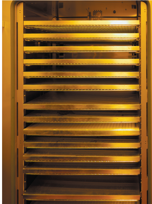
Left: Device for immersion coating the diaphragm film with photoresist – shown without cuvette and film. The coated film is tempered in heating cabinets (right), each of which has its own temperature sensor. By the way: Nothing is wrong with the white balance in these and the following photos – rather, all work related to the undeveloped, UV-sensitive photoresist is carried out in yellow light, which contains no short-wave parts that could pre-expose the resist layer.
