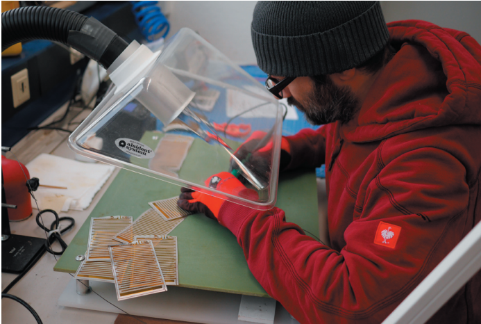
Soldering the connecting cables to the aluminum strip conductor
